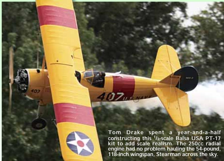
Tom Drake spent a year-and-a-half constructing this  $\frac{1}{3}$ -scale Balsa USA PT-17 kit to add scale realism. The 250cc radial engine had no problem hauling the 54-pound, 118-inch wingspan, Stearman across the sky.
