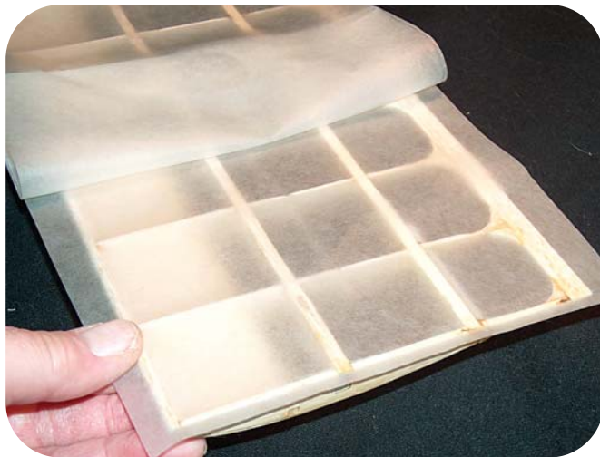
Above right: This is the top surface, but that's okay. The sheet of covering has been water-sprayed, laid smoothly in place over the wing panel, and then folded back to allow the author to dope the first section of the structure to which he wants the silkspan to adhere. It's usually best to begin at the wing root, as shown.
