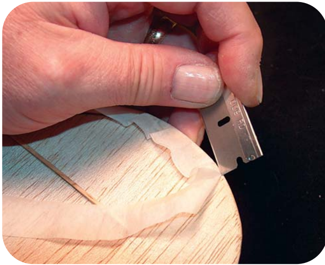
You can trim the silkspan along the back side of a curved surface, such as a wingtip, using a sharp blade and a delicate touch. Don't cut the wood!
