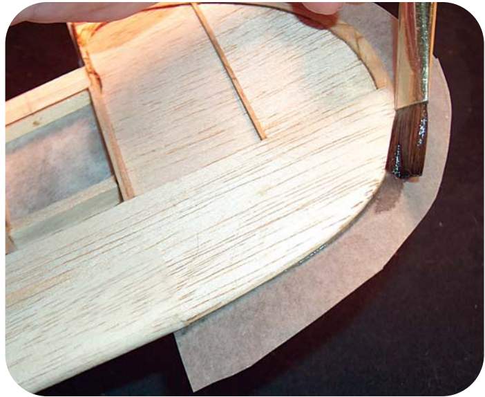
This is the back side (top surface) of the wingtip. Get plenty of fresh dope on the places where the silkspan is going to stick.
