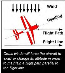
The aircraft attitude is defined as the position of the aircraft in the sky, and is characterized by the variations it has on the yaw, pitch, and roll axis. In a "no-wind" and normal speed condition, the aircraft's attitude (its heading) will generally point in the same direction as the flight path. In case of a cross wind, the aircraft attitude must vary (on the yaw axis) in order to maintain a constant and straight flight path, as required by the Scale Aerobatics rules (Fig. 2).
