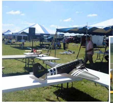
Ed Mason's DC-3 built from the Top Flite RC kit has electric power, flaps and 2.4GHz for the controls during static judging for Authentic Scale.
