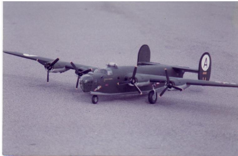
In 1988, I took a Stafford B-24 to the worlds and we placed second as a team. It had 4 OS 25s for power, rotating gun turret, retracts, flaps. What a pull in had. It weighed 14 lbs.
