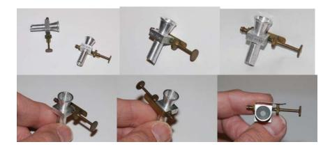
Photos of Walt Hughes' "stunt carburetor" that he developed, produced, and sold, made to fit various engines, in the early 1950s. Machined of aluminum and brass, this device was intended to provide improved stunt flying performance from the engines of the day. With its upper and lower taper, and the location of the fuel inlet, Hughes claimed this better performance.
