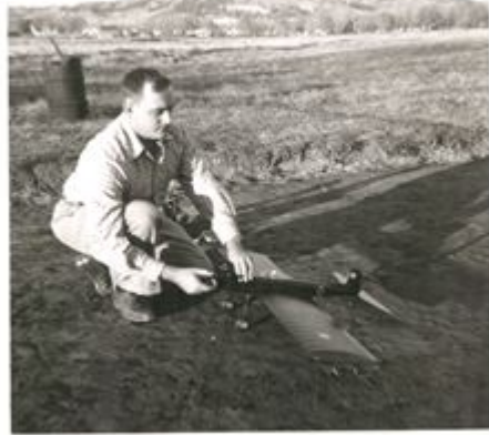
Bob's new airplane, named Von Goblin, a stunt/combat model with a KB .29 engine and 49 inch wingspan.
